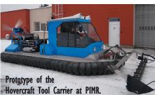
The tests of the prototype hovercraft tool carrier showed that it needed further improvement - a bigger engine (200-400kW) for its 2100 kg weight and a much deeper aircushion to give a ground clearance up to 50-70 cm. The main advantage of potentially using the hovercraft technology is that there is practically no physical impact on the protected wetlands.
