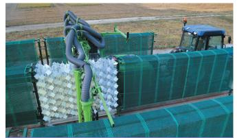
An agro-environmental test bed. This customisable artificial vine will objectively measure pesticide application by spraying during the vine's main growing stages and the evaluate the performance of various materials
