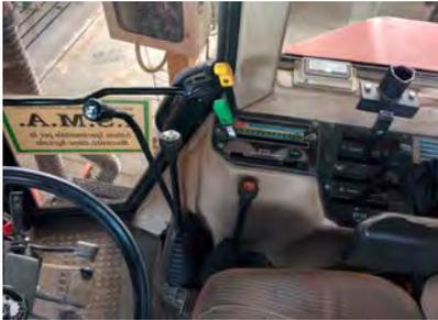
**TRACTOR 1:** transmission articulated in gears and ranges (High-Low, Rabbit-Snail).
